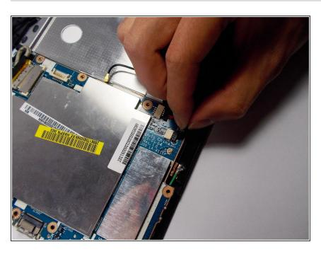
Once the microphone has been lifted away from the case, disconnect the microphone cable from the motherboard by pulling the cable out horizontally. Do not lift up to remove.
