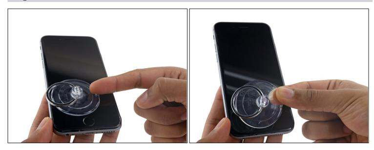
• Pull up on the nub on the top side of the suction cup to remove it from the front panel.
