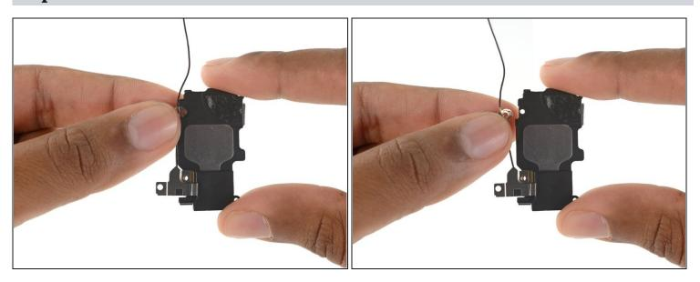
• Remove the cable clip from the left side of the speaker.
