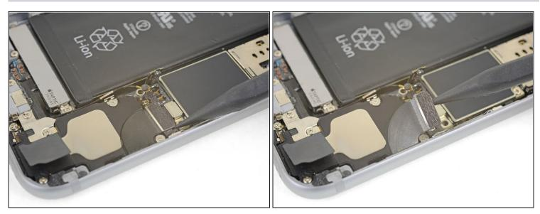
• Use the point of a spudger to lift up and disconnect the Lightning connector ribbon cable from its socket on the logic board.
