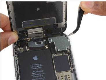
• Remove the display cable bracket.
