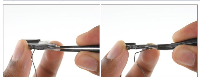
• Remove the tape covering the antenna cable on the edge of the speaker.
