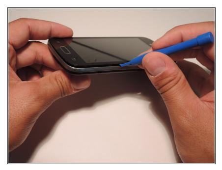
Us the plastic opening tool to pry apart the screen from the plastic.
