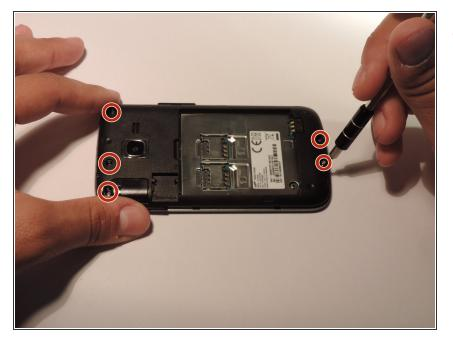
After following how to remove the battery, unscrew the five 1.2mm
