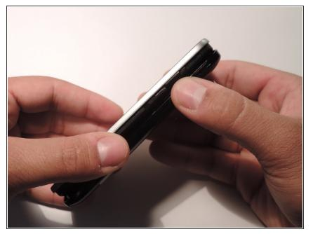
Place phone firmly between both hands with one hand flat on the back of the phone and pop off the back cover
