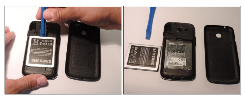
• Once rear cover is off use small pastic spudger to lift battery out of the phone
