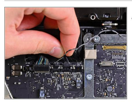
Disconnect the hard drive fan by pulling its connector toward the top edge of the iMac.
