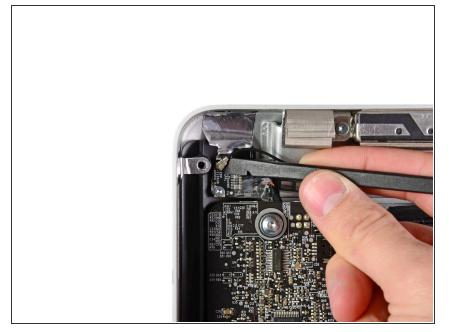
• Use the flat end of a spudger to pry the Bluetooth antenna cable connector up from its socket on the Bluetooth board.
