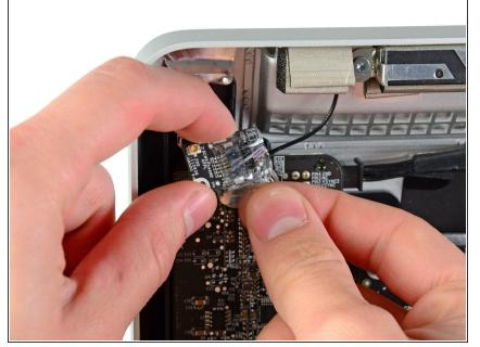
• Remove the piece of tape wrapped around the Bluetooth board.
