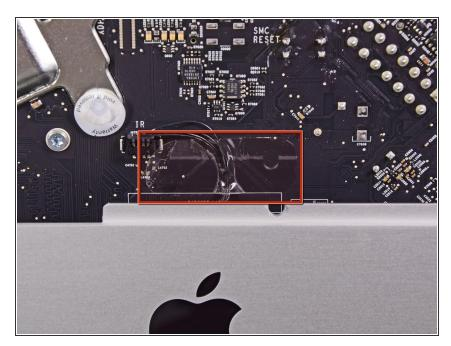
Remove the piece of tape covering the IR sensor cable.
