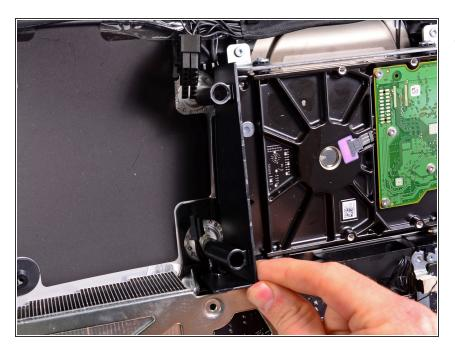
Remove the plastic pressure wall installed next to the hard drive.
