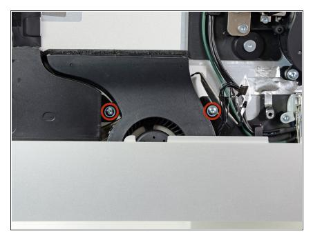
Remove the two 13 mm T10 Torx screws securing the CPU fan to the outer case.
