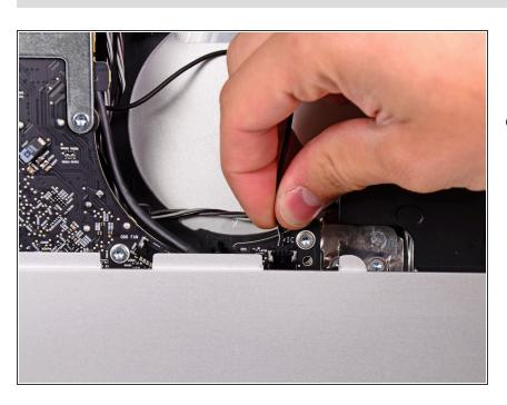
Pull the microphone cable connector toward the top edge of the iMac to disconnect it from the logic board.
