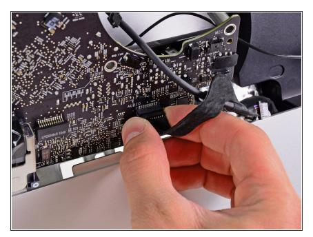
Disconnect the audio port cable by pulling its connector away from the front face of the logic board.
