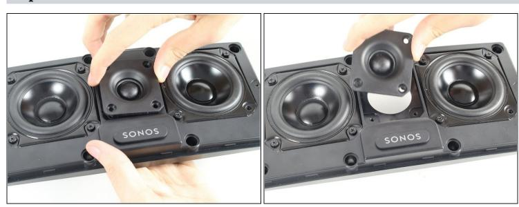
• Carefully lift the tweeter speaker out the front of the panel.
