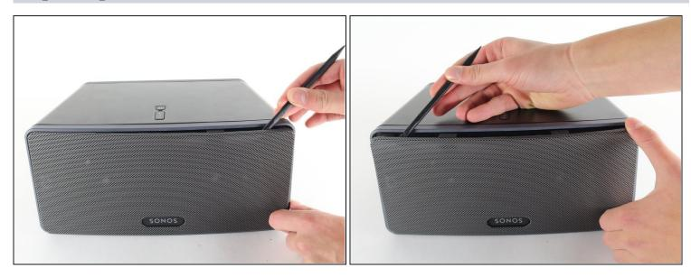
• Insert a spudger along the edge of the screen and gently use it to pull the screen away from the casing. Slide the spudger along the length of the grill to detach all the clips holding it in place.
