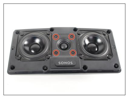
Using a Phillips #2 screwdriver, remove the screws securing the speaker to the front panel.
