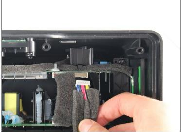
• Disconnect the front panel from the motherboard by gently reaching in and pushing the tab underneath the wire connector and pulling towards you.
