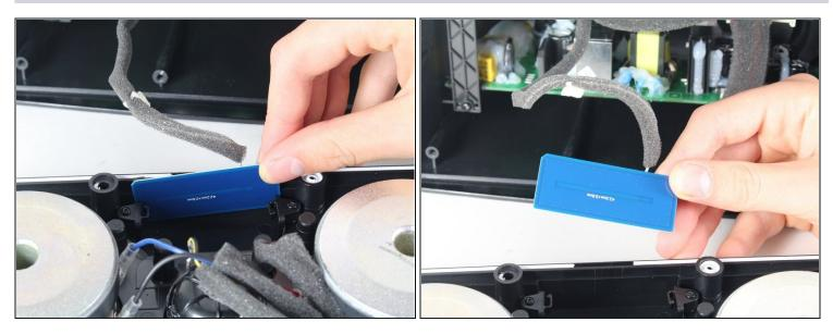
• Gently remove the wireless card located at the bottom of the front speaker panel by pulling up and out with your index finger and thumb.
