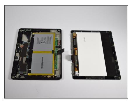
Your screen assembly has now been removed and can be replaced.
