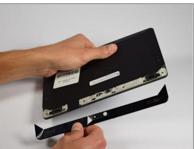
Once you reach the end of the plastic cover you should be able to completely remove it from the device.
