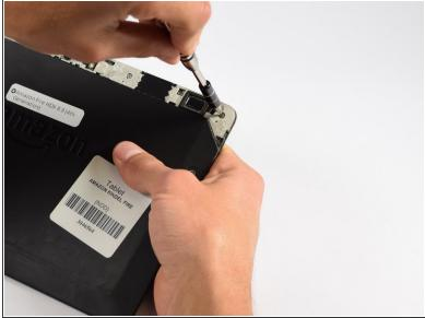
Use a T5 screwdriver to remove the four 3.5 mm T5 screws at the top of the device, where the black plastic trim was located.
