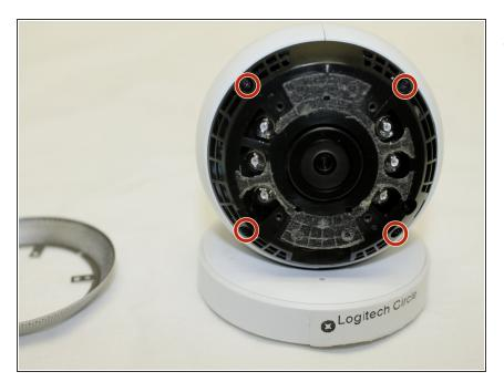
Remove the next ring by continuing to unscrew the screws in the circled locations.
