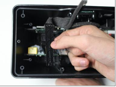
Remove the two plastic panels on either side of the device that hold the motherboard and power supply board in place.
