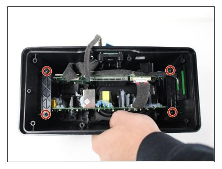
Using a Phillips #2 screwdriver, remove the 4 screws securing the two plastic panels down.
