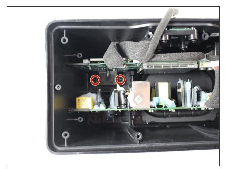
Using a Phillips screwdriver, unscrew the two screws in the back of the device that hold the motherboard in place.
