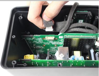
Disconnect the motherboard from the volume button board by gently grabbing the connector and pulling it towards you.
