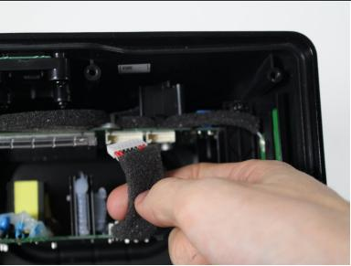
• Disconnect the motherboard from the power supply board by gently reaching in and pushing the tab underneath the wire connector and pulling towards you.
