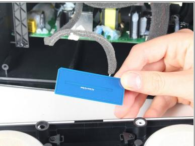
Gently remove the wireless card located at the bottom of the front speaker panel by pulling up and out with your index finger and thumb.
