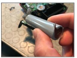
Desolder the battery leads from the PCB and remove the battery.
