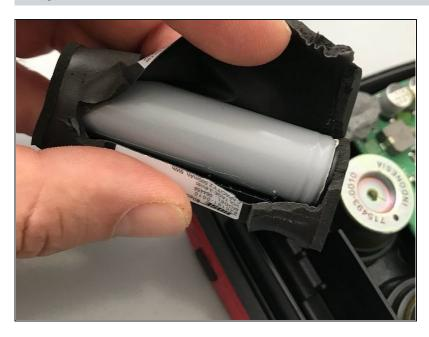
Partially cut the battery cover on the side paying attention to do not damage the circuit or the battery.
