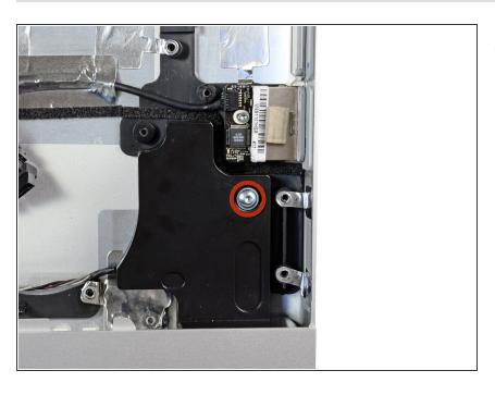
Remove the single 13 mm T10 Torx screw securing the right speaker to the outer case.
