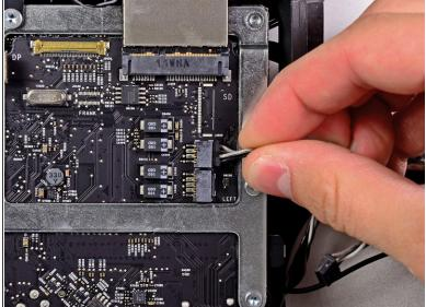
• Disconnect the left speaker and right speaker cables by pulling their connectors toward the right side of the iMac.
