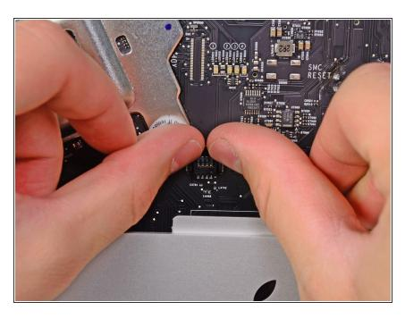
Use your thumbs to push the IR sensor connector out of its socket and toward the top edge of the iMac.
