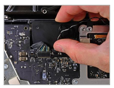
Pull the hard drive thermal sensor cable out of its socket and toward the top edge of the iMac to disconnect it from the logic board.
