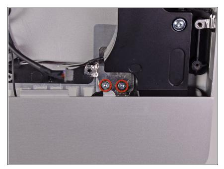
Remove two 5 mm T10 Torx screws securing the audio ports to the outer case.
