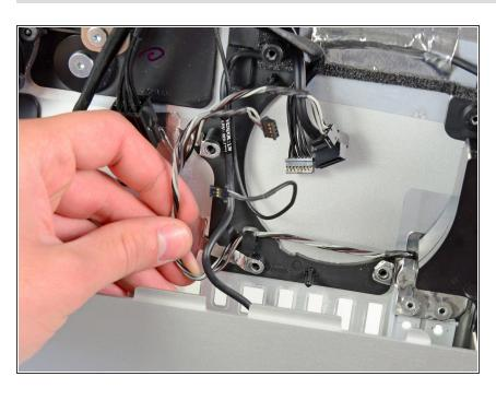
De-route the right speaker cables from the black plastic clips attached to the outer case.
