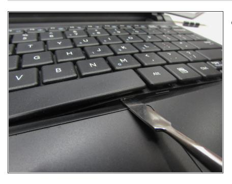
Flip the computer over. Then, use the plastic opening tools or spudger tool to push in the four, plastic tabs located at the top of the keyboard.
