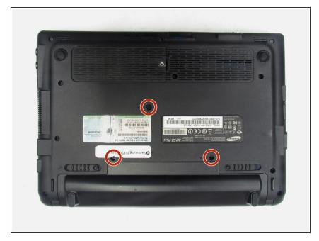
Double check that you removed the three 7mm screws for the keyboard in the process of removing the back panel
