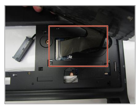
Remove the keyboard completely from the bezel and locate the ribbon cable that connects the keyboard to the motherboard.
