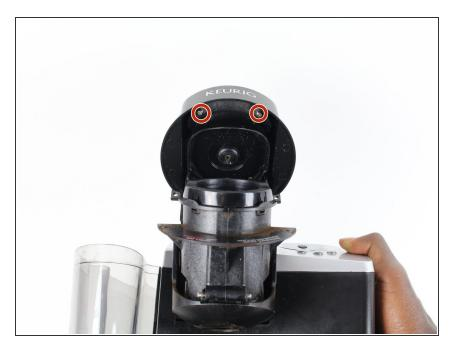
Remove the two 9.5 mm Phillips #1 screws on the underside of the lid.
