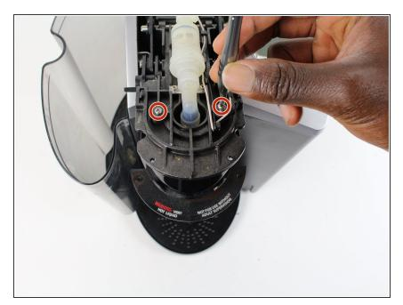
Locate and remove the two 9.5 mm
