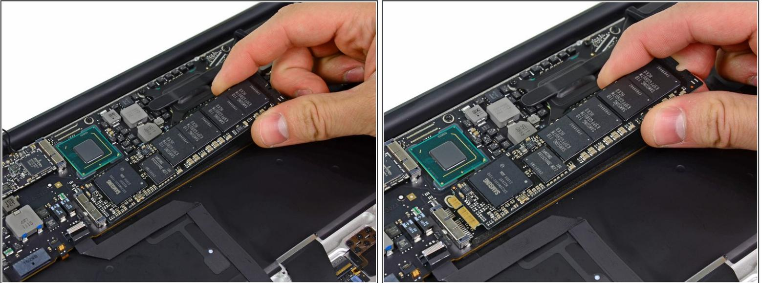
**⚠** To avoid damaging its socket, do not lift the end of the SSD excessively.
