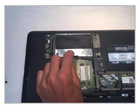
Pull out the tab to remove the hard drive.
