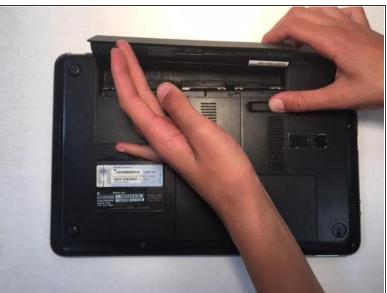
Unlock and remove the battery pack.
