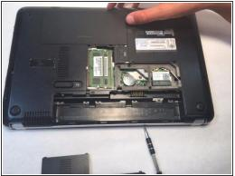
Unscrew the hidden screws covered by the battery pack and remove the panel to find more hidden screws.
