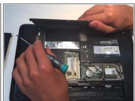
Unscrew the hidden screws in order to remove the hard drive cover.
