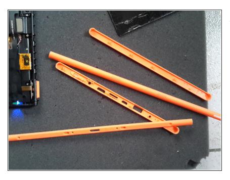
first remove the orange (or other colour) bezels from the side of the tab. the all have a small hole grip.
