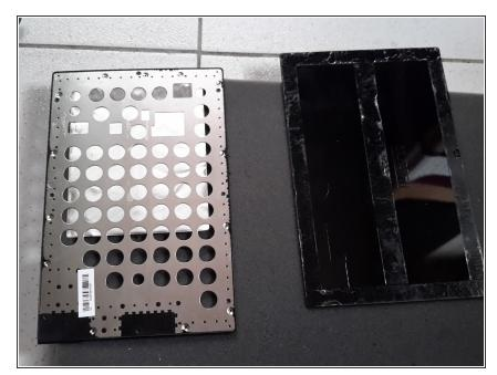
on the back cover there is a glass cover that covers up the screws. be carefull when removing it because it might break. use small like credit cards to seperate it but still be very carefull.
