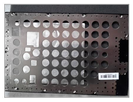
so the back cover seperates in to two parts. after removing the glass part the screws are visible. remove all of them. the back cover can pe removed very easily.
