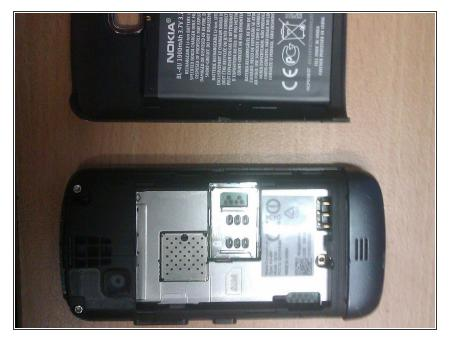
• Lift and remove the battery out of the C5's inner framework.
