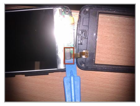
Use the flat end of a plastic opening tool to pry the digitizer cable connector up and out of its socket on the motherboard.
