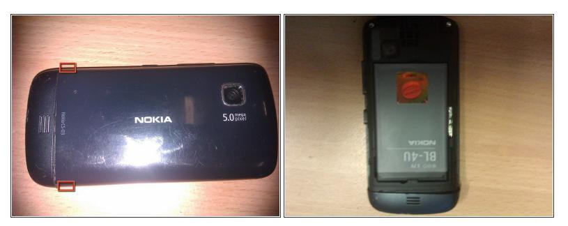
(i) There are two clips (highlighted in red) securing the rear cover to the framework of the C5.
