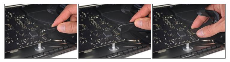
• Continuing to support the display with one hand, flip up the metal retaining bracket on the display data cable.
