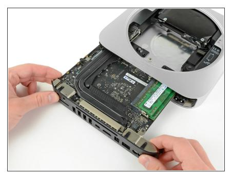
• Carefully slide the logic board assembly out of the mini, minding any cables that may get caught.
