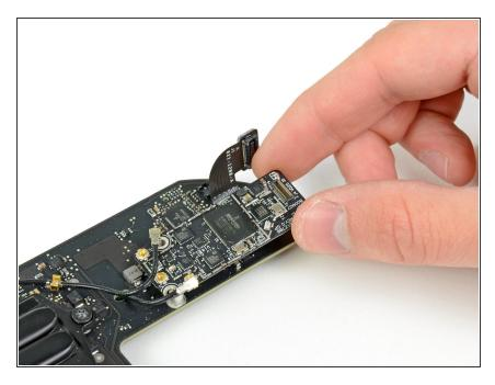
• Remove the AirPort/Bluetooth board from the logic board.
