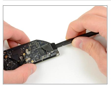
Use your spudger to help disconnect the AirPort/Bluetooth ribbon cable from its socket on the AirPort/Bluetooth board.
