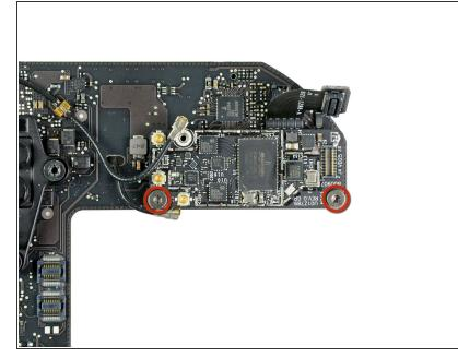
Remove the two 2.6 mm T6 Torx screws securing the AirPort/Bluetooth board to the logic board.
