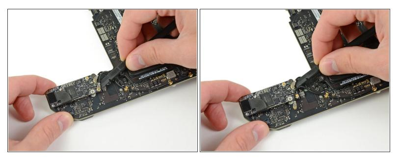
Use the flat end of a spudger to pry both antenna connectors up from their sockets on the AirPort/Bluetooth board.
