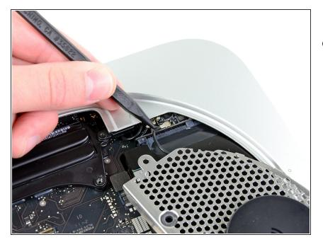
Use the tip of a spudger to carefully pry the antenna connector up from its socket on the AirPort/Bluetooth board.
