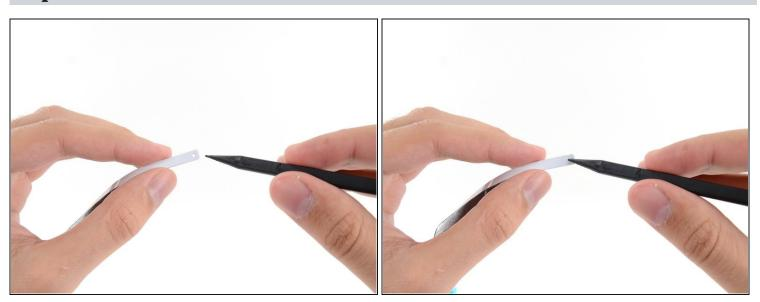
Insert the tip of a spudger into the hole at the end of the strip from the side that still has a backing on it.
