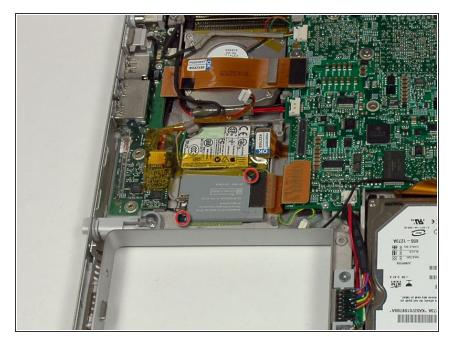
Remove the two Phillips screws holding the Airport Extreme/Bluetooth card to the lower case.
