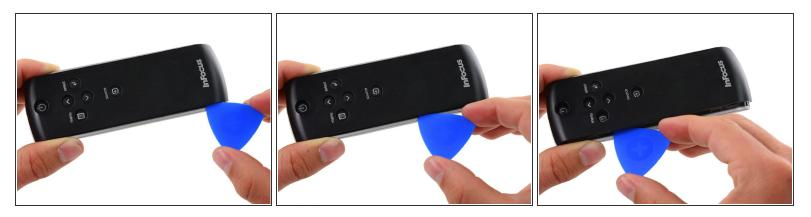
• Repeat the previous step on the other side of the remote, working from the InFocus label towards the buttons until the entire cover is loose.
