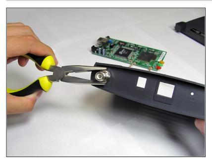
Using a pair of needle nose pliers, remove the nuts that secure the antenna ports to the rear panel.
