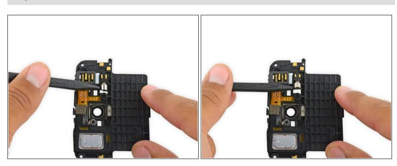
• Use the pointed end of a spudger to gently pry the vibrator up and away from the midframe.
