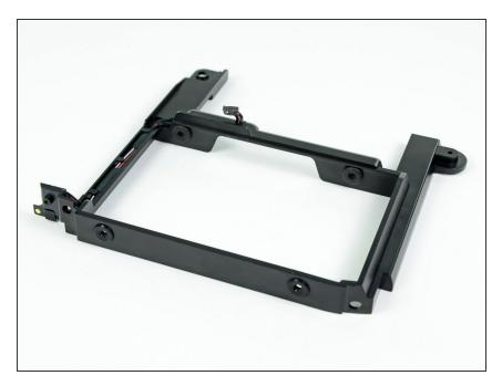
The bracket with all four grommets installed should look like the bracket shown in this picture.
