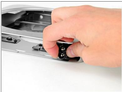
Rotate the AC-In connector 90 degrees counter-clockwise.
