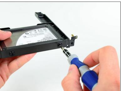
Use a T6 Torx screwdriver to install the remaining two set screws through the grommets and into the side of the hard drive.
