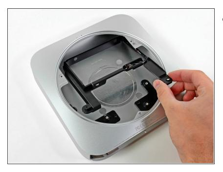
Remove the hard drive tray from the outer case.
