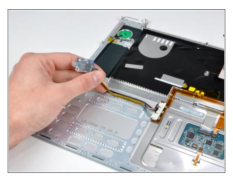
Peel up the Bluetooth data cable from the adhesive on the upper case, removing tape as necessary.
