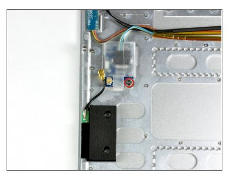
Remove the single Phillips screw securing the Bluetooth board to the upper case.
