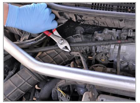
• Use a pair of pliers to slide the hose clamp off the tube attaching the valve cover breather to the air intake hose.
