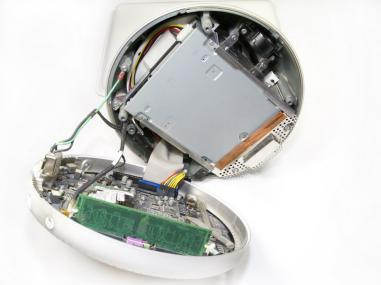
• Open the base by carefully pulling straight off, do not rotate the cover.
