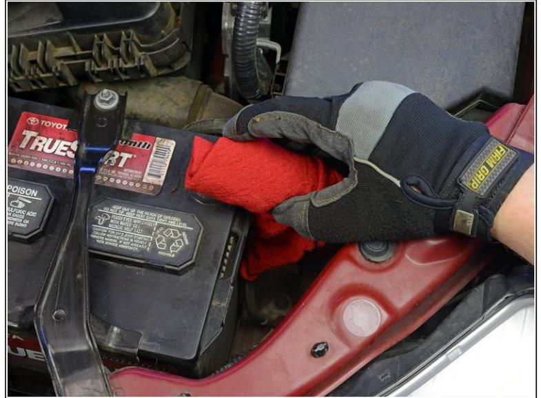
**⚠** Prevent the cable from making accidental contact with the terminal by pushing it aside and/or wrapping the cable clamp with a dry rag.
