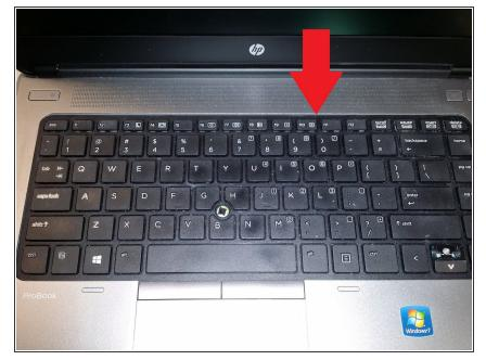
Take a spudger tool and pry the keyboard down toward the mouse pad and up toward you. After you raise the keyboard there are tabs at the bottom. Pull the keyboard away from you, and it will dislodge.
