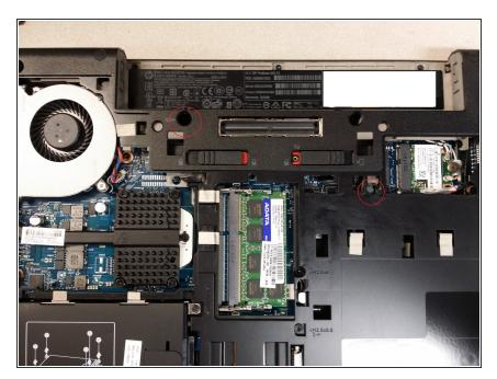
Remove the two screws at the two indicated locations with the phillips head screw driver.
