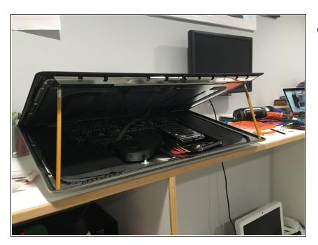
The current iFixit and OWC guides have you disconnect the display cables, with this guide you don't need to. I kept my iMac horizontal and after opening the display I simply used two standard pencils to prop up the display on both sides.
