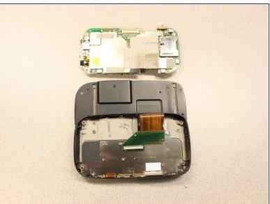
Remove the flexible connection from the motherboard.
