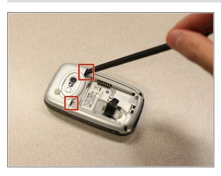
Insert the flat end of the <u>spudger</u> into the two notches on the back of the camera cover and pry them up.
