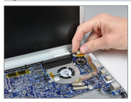
Remove the foam bumper from the top of the right hinge of the display.
