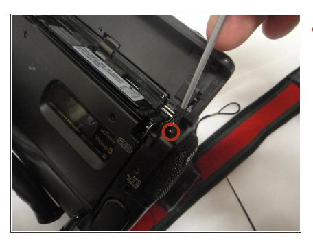
Remove the Phillips #00 screw holding the microphone on.
