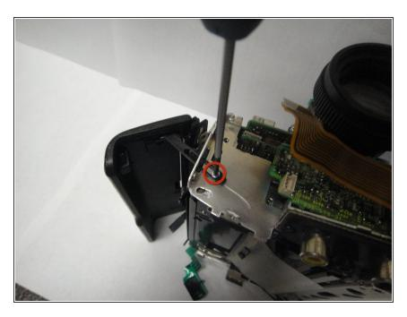
Remove the Phillips #00 screw from the tape transport slider.
