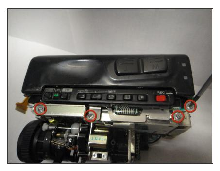
Remove the four Phillips #00 screws located on the top of the camera.
