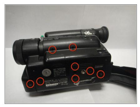
Remove the eight Phillips #00 screws. There are six screws on the bottom of the camera and two screws beneath the back light button.
