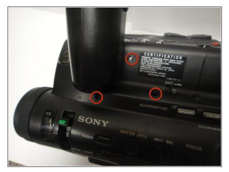
Remove the three Phillips #00 screws located on the top of the lens side cover.
