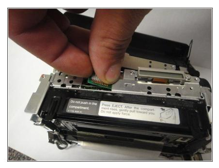
Remove the electrical connector from camera.
