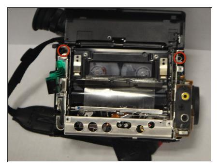
Remove the two Phillips #00 screws from lens side cover.
