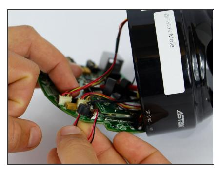
Gently pull back the motherboard to expose many of the component's wired connections.
