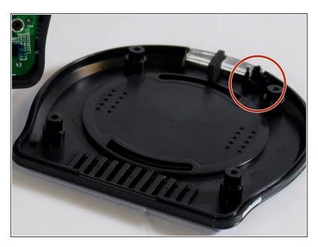
• Remove microphone from its holder on the bottom section of the casing.
