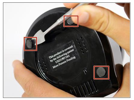
• Remove the four bottom tabs in order to access the bottom screws.
