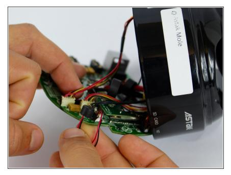
Gently pull back the motherboard to expose many of the component's wired connections.
