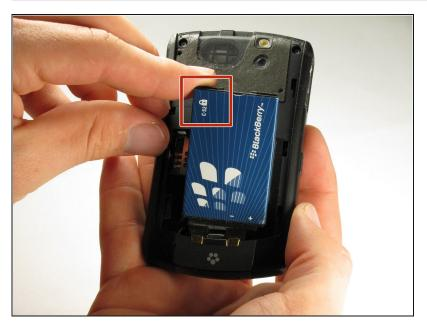
Pull up on the top edge of the battery to remove it.
