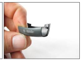
• Use a plastic opening tool to gently pry the bottom cover loose.
