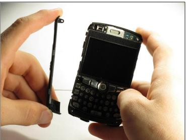
• After the bottom two screws have been removed the side casings can be removed.
