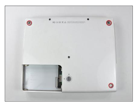
Remove the three newly-revealed Phillips screws.
