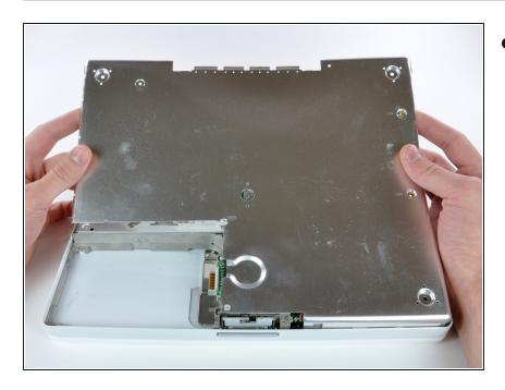
• Lift the bottom shield off.
