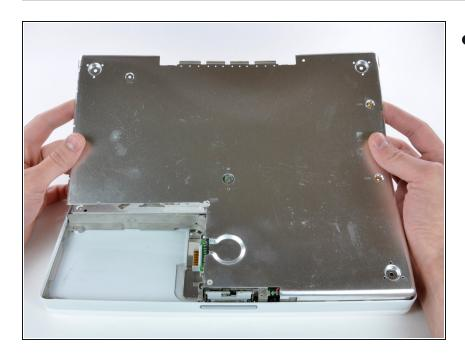
• Lift the bottom shield off.
