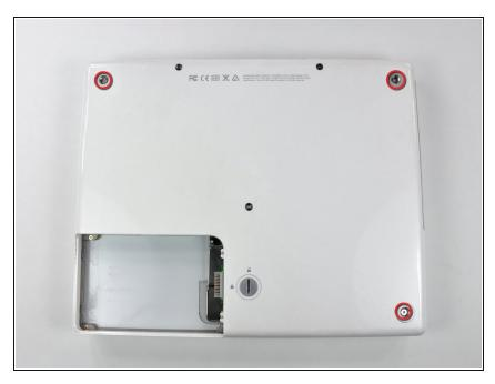
Remove the three newly-revealed Phillips screws.
