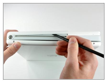
There are three tabs over the optical drive that must be released before the lower case can come off. Slide the spudger into the lower case above the optical drive and run it toward the back of the computer until you hear three distinct clicks.
