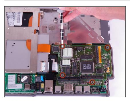
Use T8 torx screwdriver to remove four, 7.7mm long screws from the perimeter of the daughterboard.
