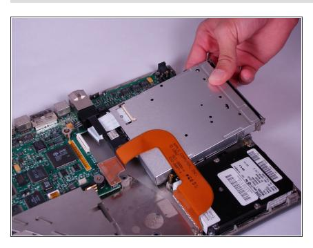
Lift the floppy drive upwards to remove it.
