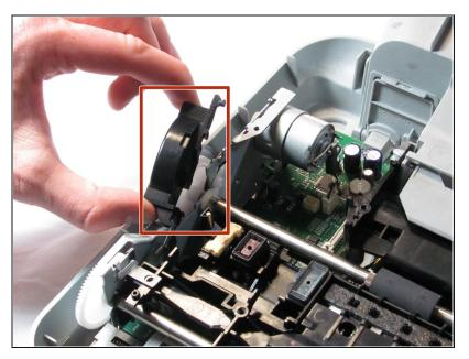
• Remove the plastic gear cover by pulling it away from the printer body and lifting it up.
