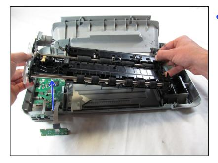
• Lift the feed roller assembly straight up to remove it.
