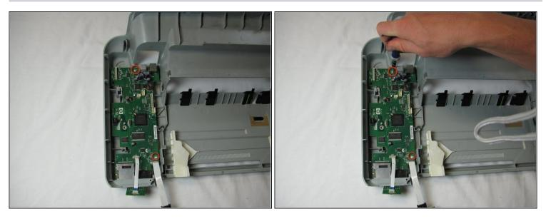
• Remove the two T10 12mm Torx screws from the main circuit board.
