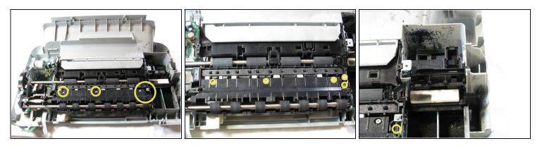
• Remove the five T10 12mm Torx screws from the roller holder.
