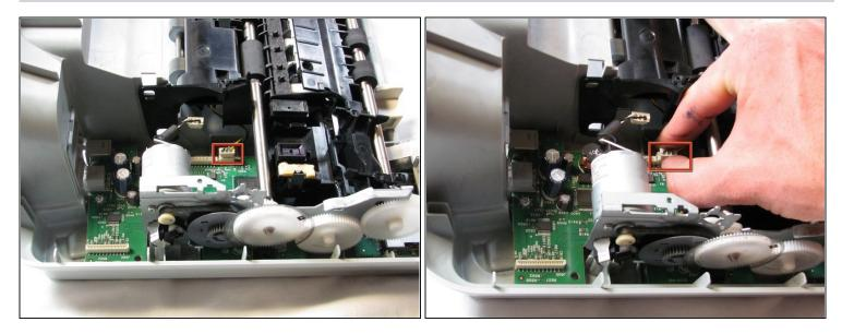
• Disconnect the page sensor from the logic board by pulling straight up on the connector.
