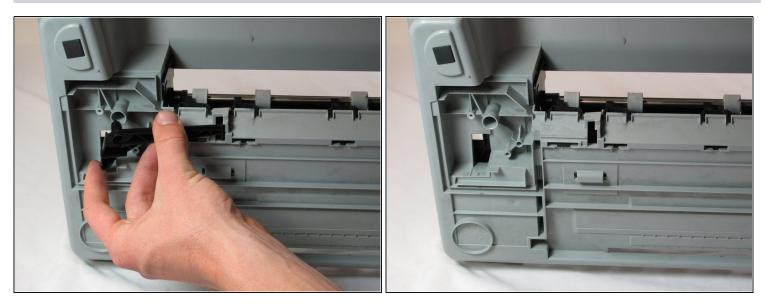
• Remove the black plastic cross member from the bottom of the printer.
