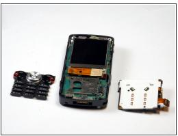
Insert the plastic opening tool under the ribbon cable attachment and give a small push upwards to dislodge it.
