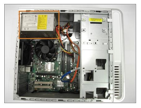
• Locate the power supply in upperback corner of the case.
