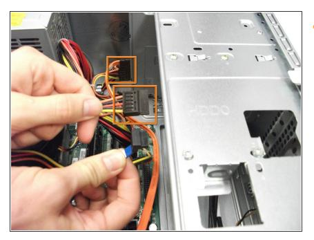
Remove the power cables from the CD/DVD drive and hard drive.
