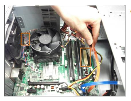
Remove the two power cables from the motherboard.
