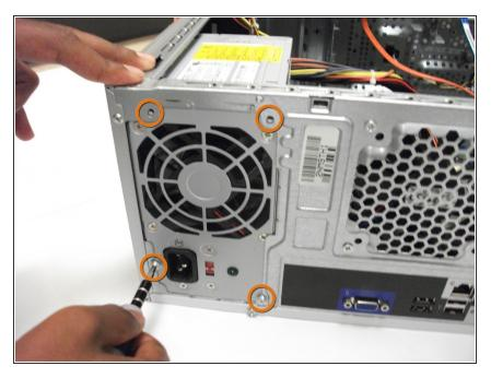
Locate and remove the four Philips #0 8.9 mm screws on the outside of the case.
