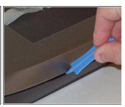
• Push the plastic opening tools into the crack between the top and the bottom of the chassis.
