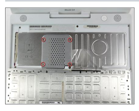
Remove the four silver Phillips screws that secure the RAM shield.
