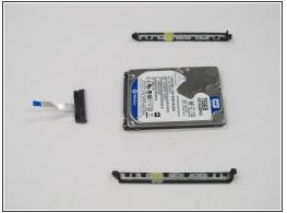
Pull the rubber casing away from the hard drive.
