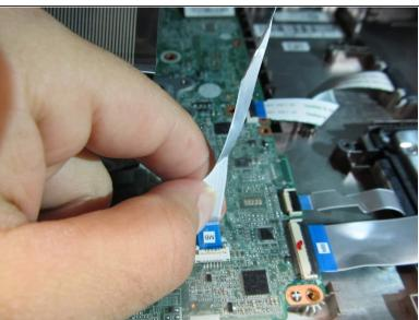
Remove the ribbon connecting the mousepad to the motherboard.
