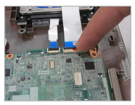
Lift the black retaining bar that holds down the two hard drive ribbons to unlock them.
