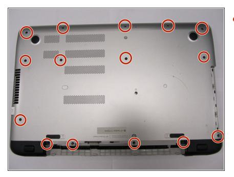
Remove fifteen 7 mm screws with a Phillips #1 screwdriver.
