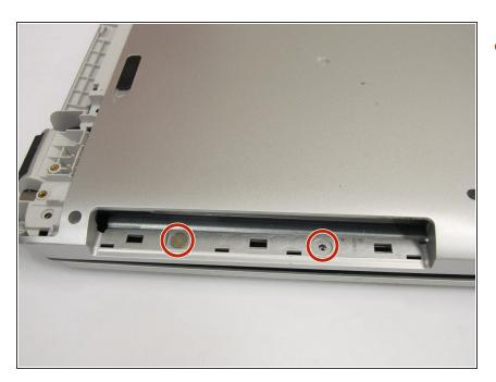
Remove two 2.4 mm broadhead screws from the CD Drive bay with a Phillips #0 screwdriver.
