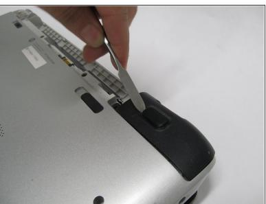
Use a metal spudger to remove the rubber "feet" to expose two screws.
