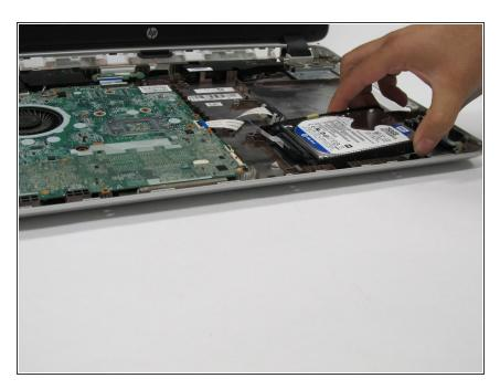
Lift the hard drive out from the enclosure.
