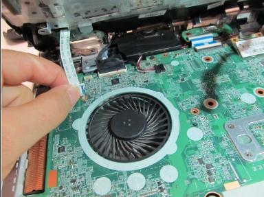
Remove the ribbon connecting the power button to the motherboard.
