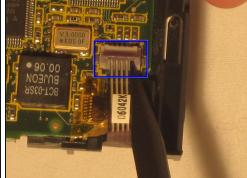
• Place the plastic screen cover back on the front of the device and reconnect the three ZIF connector tails.
