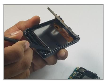
Using the spudger lift up the LCD screen and replace with the new screen.
